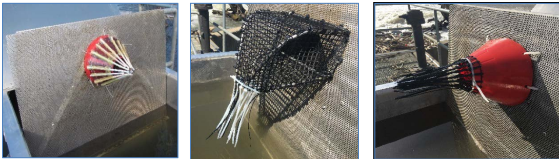
Photo 5. Examples of fyke designs that were successful in funneling lamprey to the trap box (the hinged fyke plate is lifted to show the hole end of the fyke design). An 8.25" diameter funnel with drinking straw extension (left photo). An 8.25" diameter funnel with zip tie extensions (center photo). A metal frame with vexar plastic covering and zip tie extension (right photo); this design was later modified to reduce the sharp angle that lamprey has to turn to enter (reduced it from 135 to 45 degrees). These designs allow lampreys to pass through while preventing those in the trap from escaping. Vexar plastic covering was also glued to the inside of the funnels to prevent lamprey from resting inside the funnel (which prevented other lamprey from accessing the hole).
